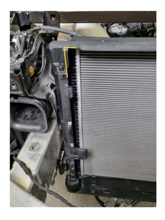
Note for step 11-18: It is possible to cut the plastic radiator supports with the front radiator air duct in place but it is a bit tight space. To have better access you can remove the front air duct by first removing the lower support beam (under bumper beam) then remove the radiator air duct.
