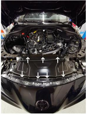
Remove the rubber seal and remove the 4 x 10mm hex holding the bumper cover.
