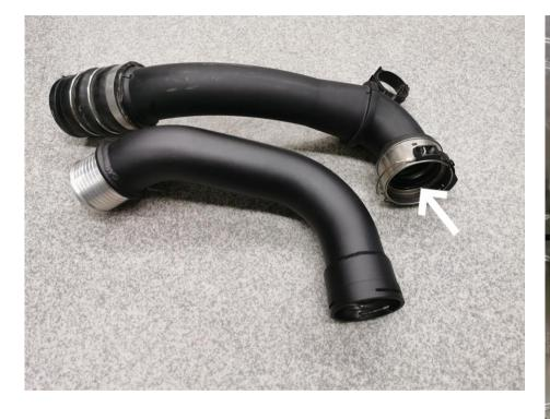
Remove the c-clip from OE pipe by prying of the plastic retainer. Then transfer the OEM sealing ring and install it and the c-clip to the do88 performance charge pipe.
