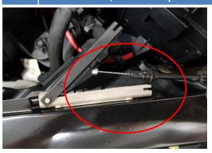
11. Remove 3x Torx T30 for the brackets above both head lights. Remove both brackets, on the left side you need to disconnect washer fluid pipe and cable hood lock joiner.
