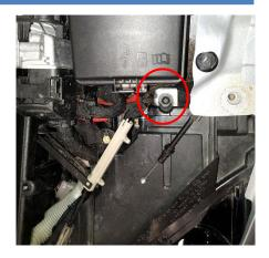
Remove the air intake scoop by removing 2x Torx T25 and disconnect the radiator hose from clips.
