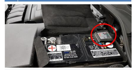
Remove 2x Torx T25 and then remove the grille. Gently pull it forward and then upwards.
