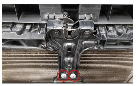
Now place a steady support underneath the radiator pack. On both sides remove 4x Hex 16mm screws and 2x Torx T30 screws. Then with the help of a friend remove the crash bar from the car.
