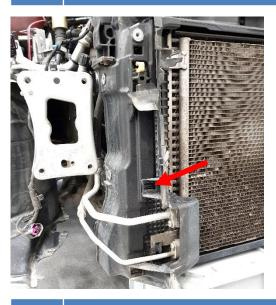
20. The intercooler and radiator assembly is fastened with the two large plastic clips. Release these with a flat blade screwdriver. Gently press the intercooler backwards while pressing on these clips.
