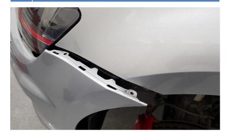
**9.** Gently lift the bumper forward a little bit, then disconnect all cable connectors.
