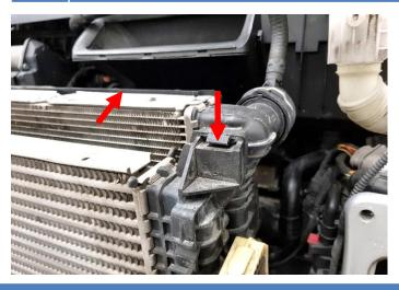
Tape the included 5mm thick sealing strip on the outside of the welding line on both sides according to the photo below. On both lower radiator brackets put a piece of the included 4mm thick self-adhesive rubber strip according to photo below. Remove the OEM intercooler brackets and install them on the do88 intercooler.
