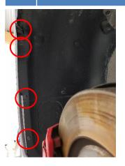
With help from a friend bend out the bumper on each side and pull it forward about 20cm and hold it in this position.
