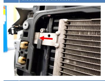
The left sides air guide needs to be slightly trimmed. Cut the plastic with a plier on the marked locations.
