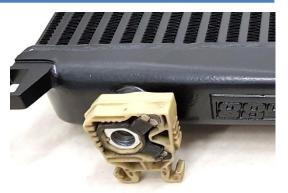
25. Cut the top right bracket on the AC-condenser. Cut on the outside of the raised rib.
