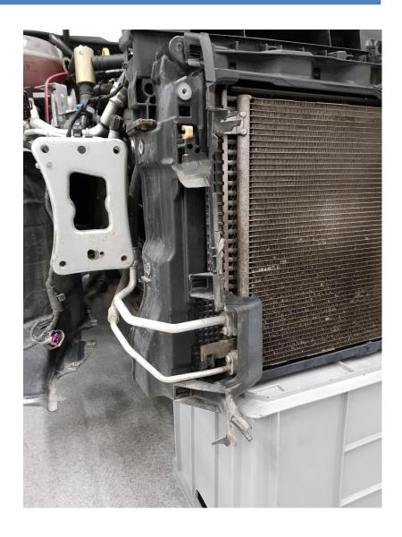
Remove the plastic air guides on both sides. Press the plastic clips downwards with a flat screwdriver.
